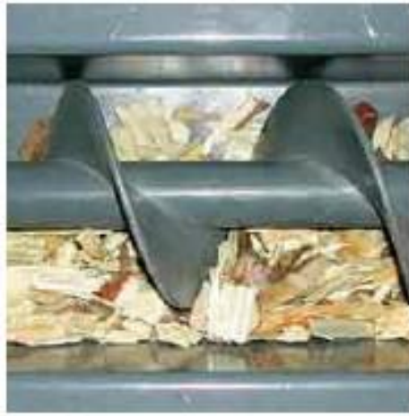
Fig 9 Wood chip auger screw
