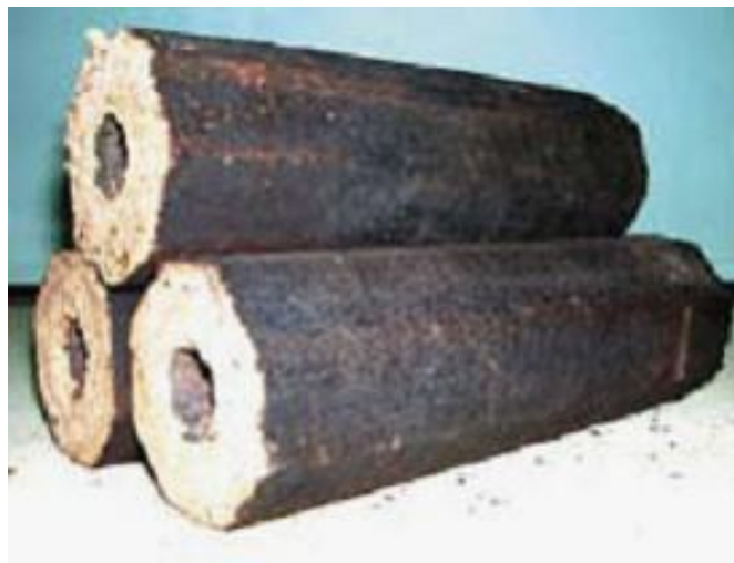
Fig 1 EFB fibre (50%) and sawdust (50%) briquette
